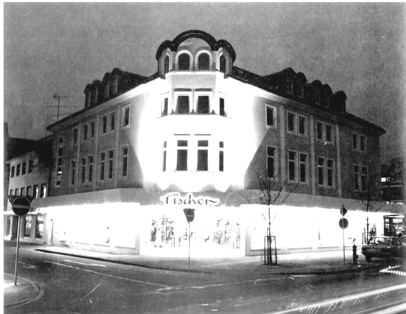
Example of corner building with demonstration of lighting techniques such as lighting of architectural features at the corners, well-illuminated store windows, and integrated canopy lighting.
