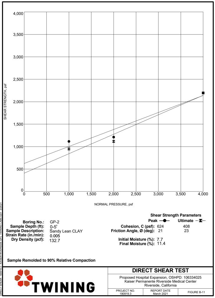
DIRECT SHEAR 190919.3 - KAISER RIVERSIDE.GPJ TWINING LABS.GDT 3/24/21
