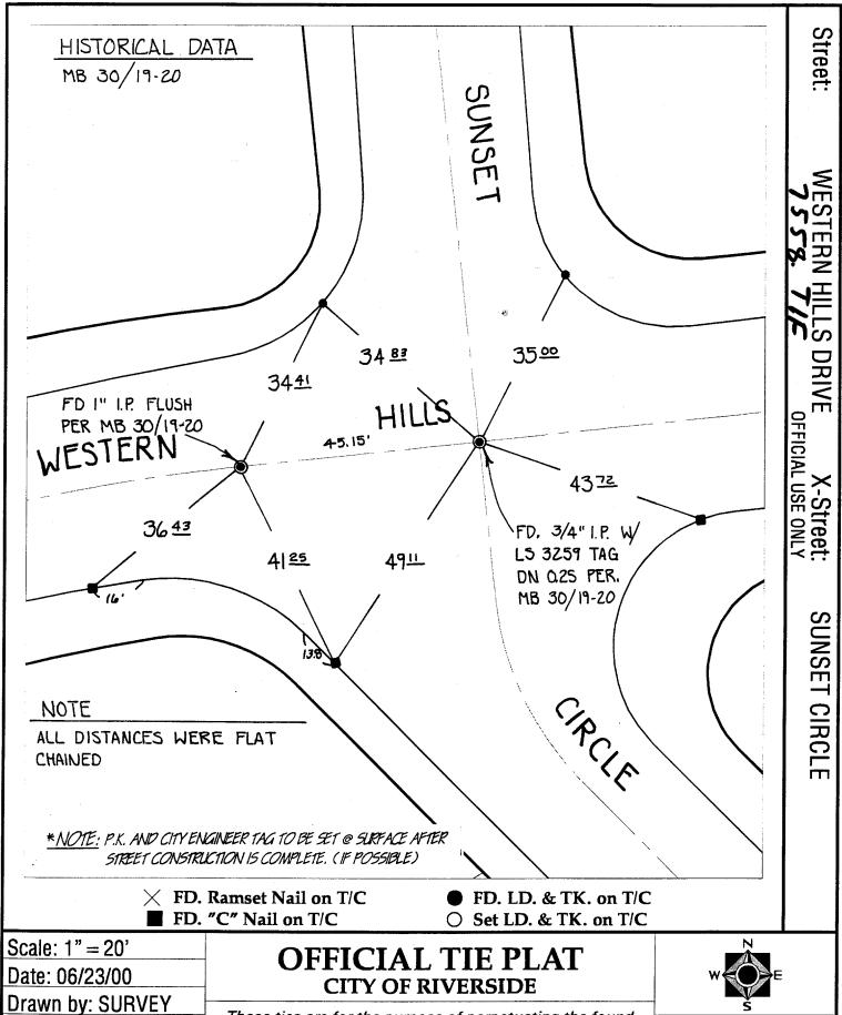
These ties are for the purpose of perpetuating the found W.O.: monumentation. No claim is made as to the relationship of F.B.: the points or lines shown hereon to true boundary locations.
