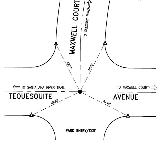
FOUND 3/4" IP OPEN W/NAIL IN CENTER DOWN 0.10', ACCEPTED AS C/L PER RIVERSIDE COUNTY TRACT No. 5347, M.B. 80/5-6, DESTROYED DUE TO CONSTRUCTION, SET GEAR SPIKE W/ WASHER "LS 3983", FLUSH.
