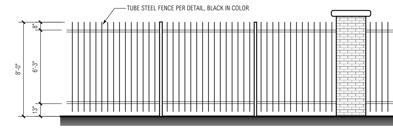
TYPICAL TUBE STEEL FENCE ELEVATION
