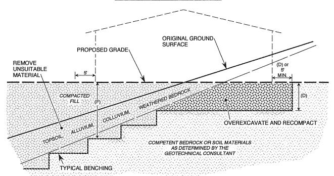
MAXIMUM FILL THICKNESS (F) DEPTH OF OVEREXCAVATION (D)
