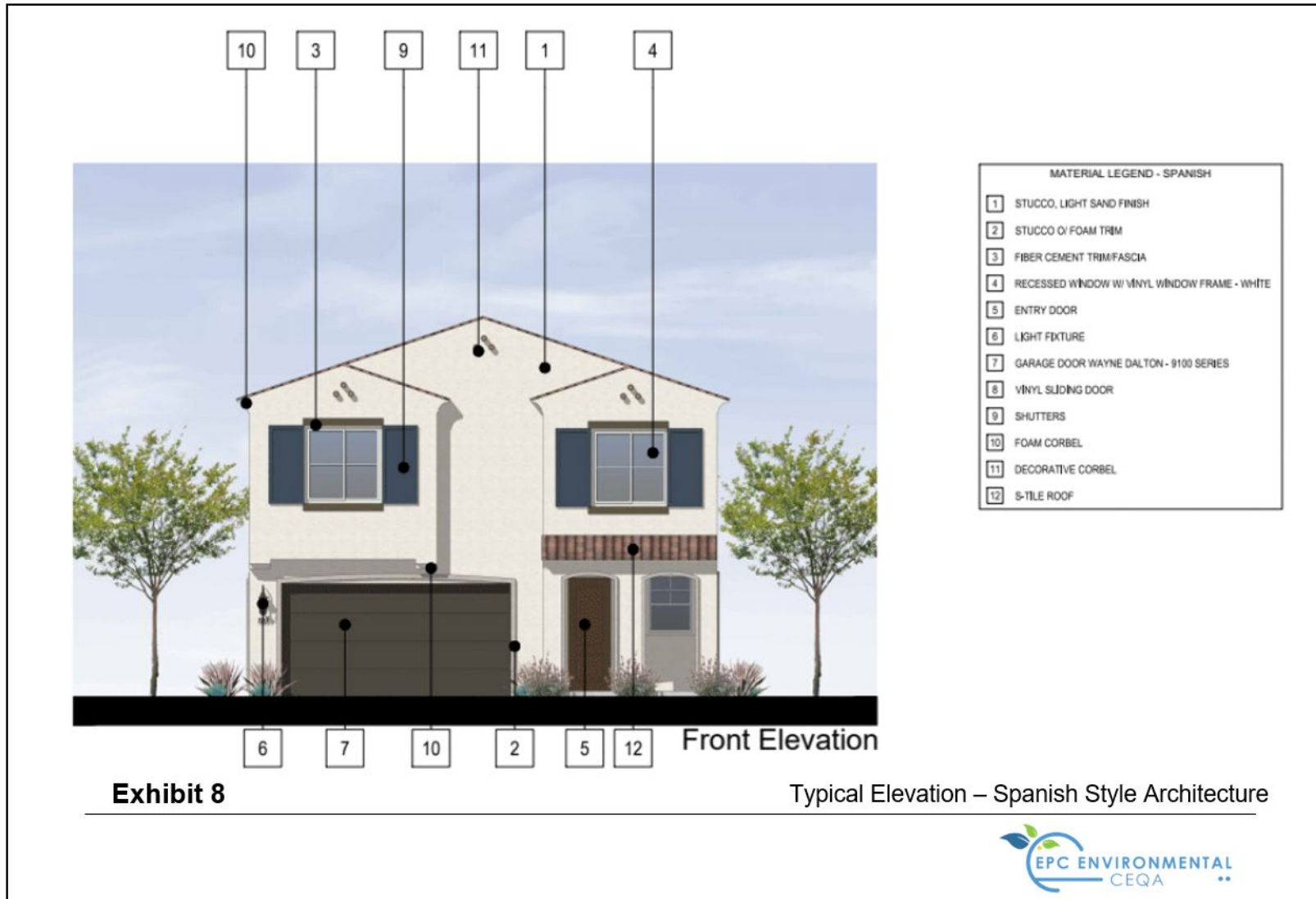
Figure 8- Typical Elevation- Spanish Style Architecture
