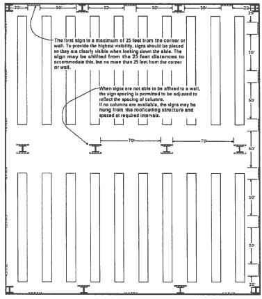
FIGURE 17 - SIGNAGE PLACEMENT AND SPACING EXAMPLE
