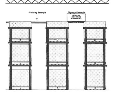
FIGURE 18 - END OF AISLE VIEW OF SIGNAGE AND STRIPING PLACEMENT EXAMPLE
