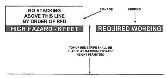
FIGURE 15 - SIGNAGE AND STRIPING VERTICAL INSTALLATION EXAMPLE
