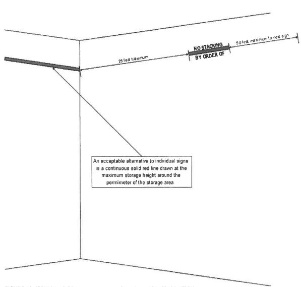
FIGURE 16 - ISOMETRIC CORNER EXAMPLE FOR MARKING INSTALLATION
