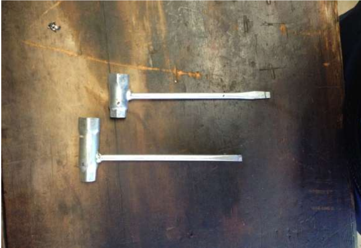
Scrench: Combination of a socket wrench and a flat head screwdriver
