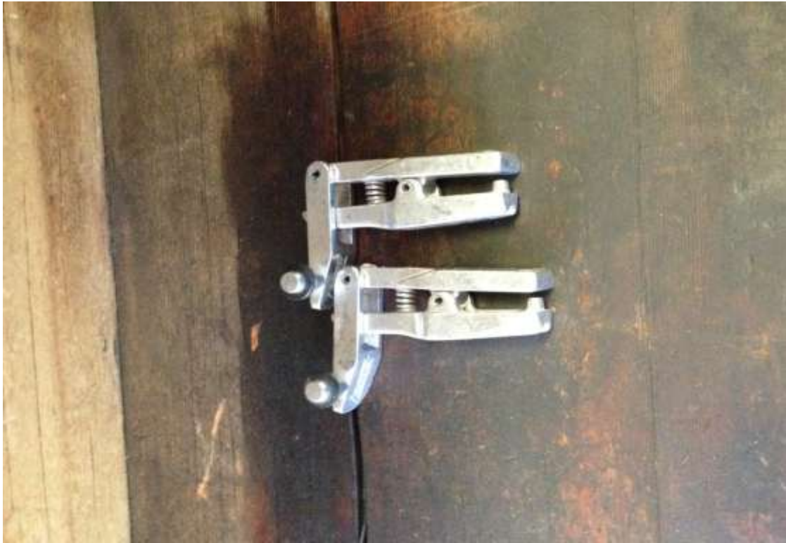
Sprinkler Shut Offs
