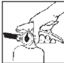
Squeeze the lever on the fire extinguisher.
