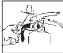
Place the extinguisher on the floor. Hold it by the tank (pressure on the handle could pinch the pin). Pull the pin straight out.
