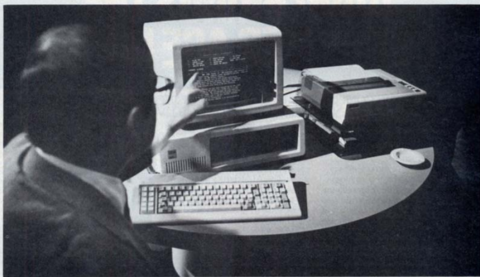
The IBM personal computer (Box 1328, Boca Raton, Fla. 33432) can be made into a complete system by adding the disc drives and printer as shown here. Other options, such as memory and graphics, are added with internal circuit boards.
