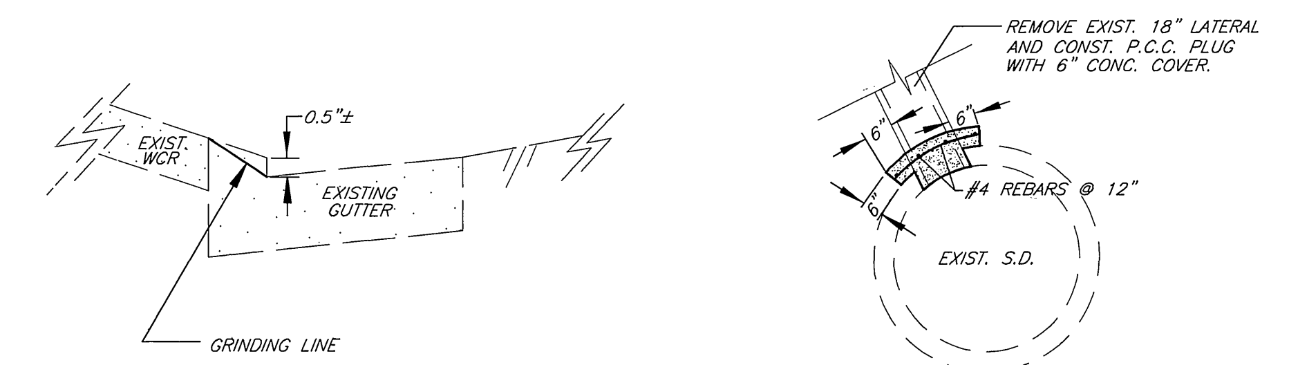
WCR CURB FACE GRINDING DETAIL
