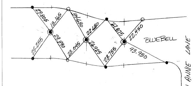
× FD. Ramset Nail on T/C ● FD. LD. & TK. on T/C FD. "C" Nail on T/C
