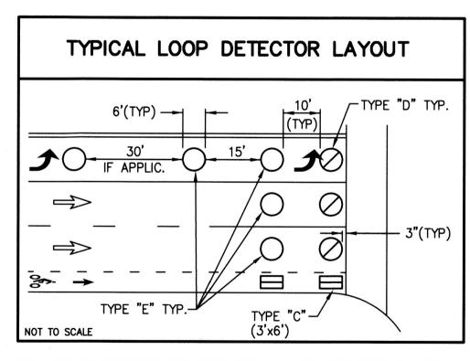
SEE CITY OF RIVERSIDE STANDARD DWG NO. 670 FOR TYPE "D" AND TYPE "C" LOOP CONFIGURATION
